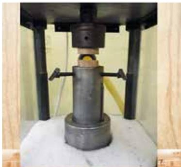
*Rotational wood welding machine holders*
