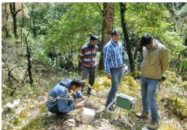
*Measurement of soil CO<sub>2</sub> efflux rate at study site*
