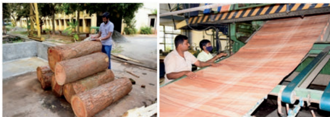
Manufacture of face quality veneer from plantation grown Meliadubia
